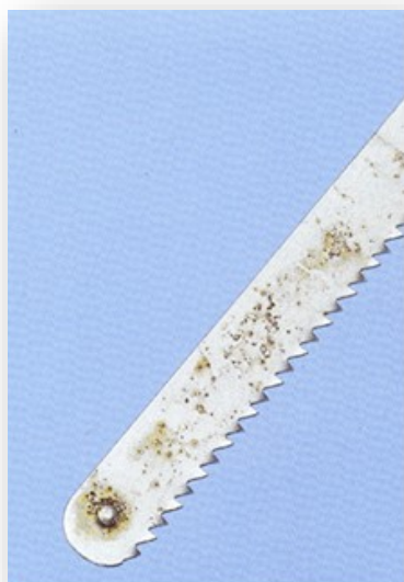
Figure 15: Discolouration and Rusting due to poor cleaning
