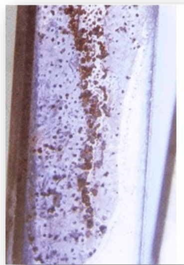
Figure 17: Pitting due to Caustic Solution—magnified
